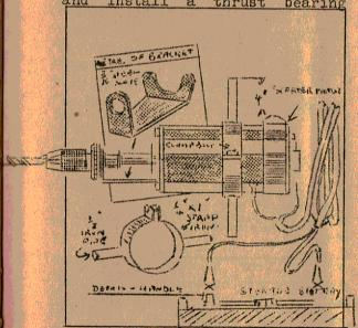
and drill chuck in its place. As there is considerable pressure on the drill, when drilling heavy metal, the thrust bearing is very necessary. The chuck mounting of course, must conform to the particular requirements of the starter you may happen to be using. The sketch shows how to mount the handles. If the motor revolves in the wrong direction, the connections to the filed coils must be reversed.
